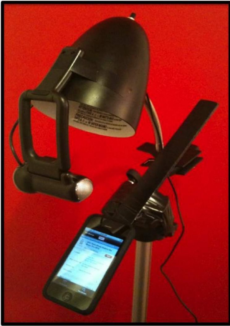
Figure 6-3. Meetup's mobile usability testing rig.
